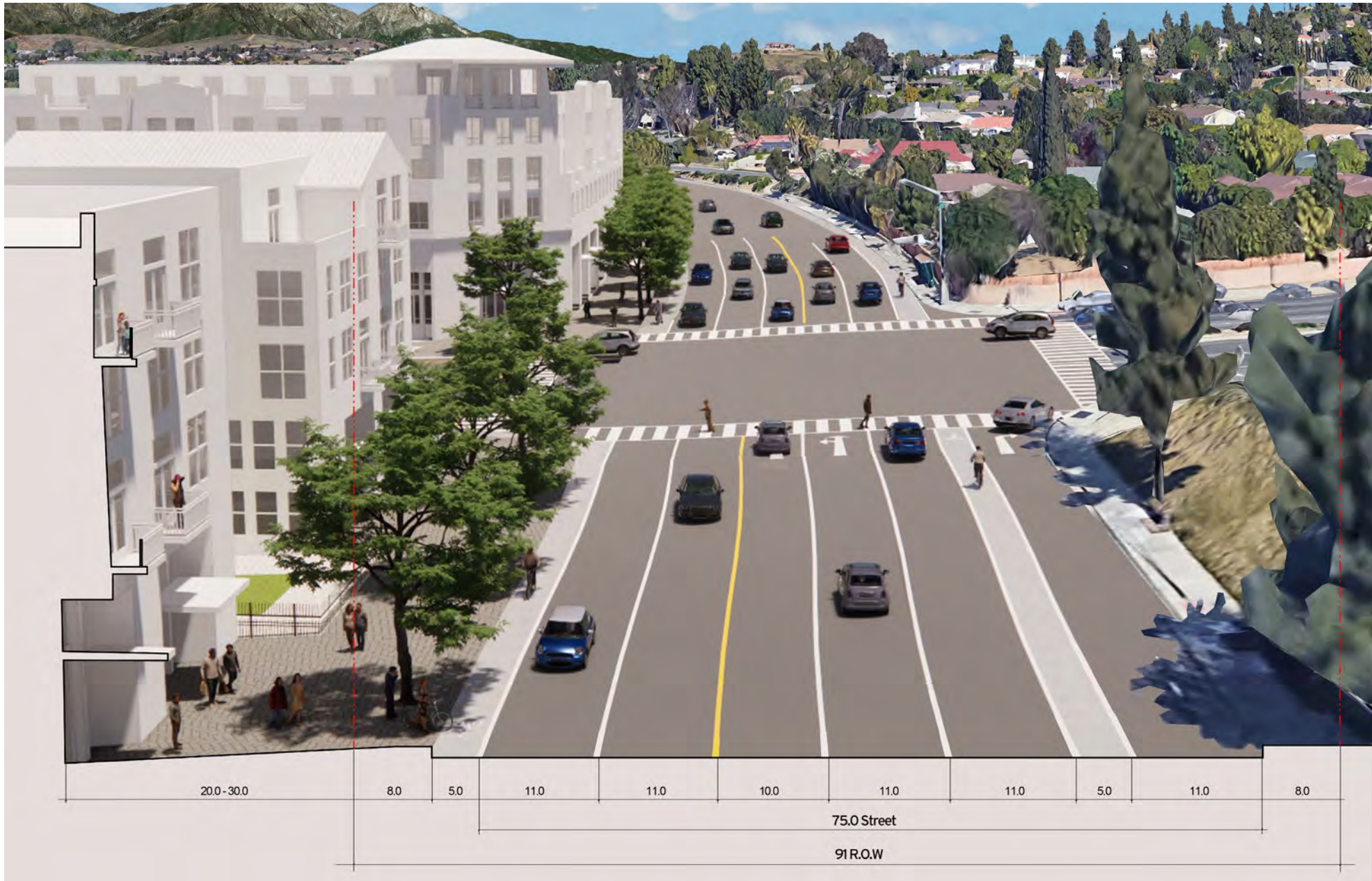
Figure 3-16 - Re-configured Golden Springs Drive street section
