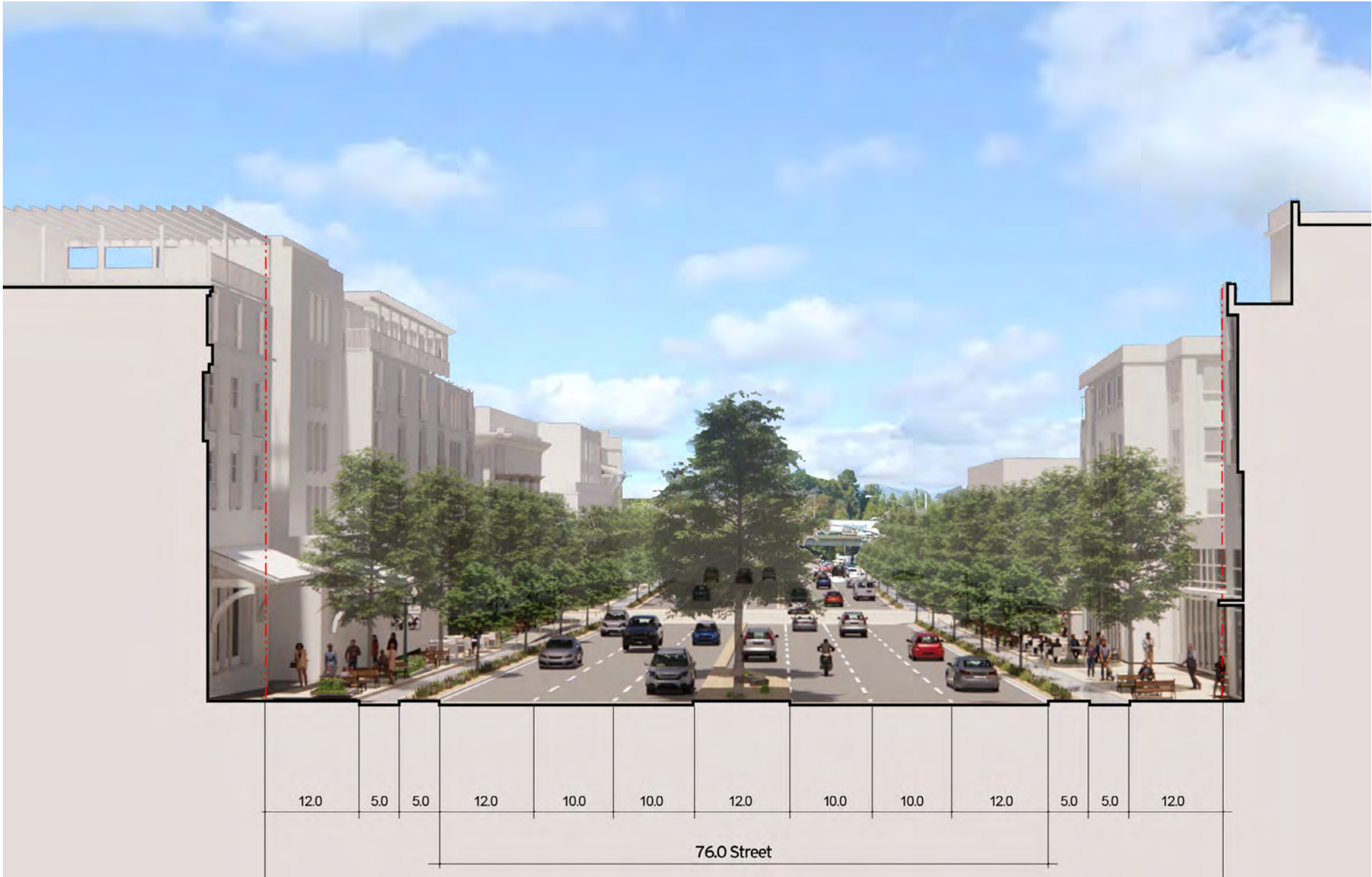
Figure 3-12 - Re-configured Diamond Bar Boulevard street section
