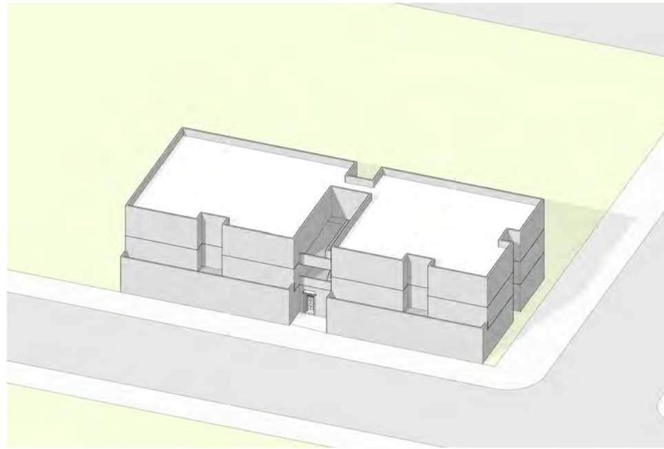
Figure 6-16 - Walk-Up Building Diagram A grouping of units around a central stair entrance.
