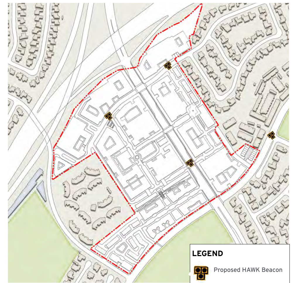
Figure 3-6 - New Traffic Signal and HAWK Beacon Locations
