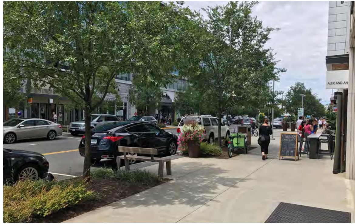
Figure 6-65 - The Storefront Activity Zone is the space closest to the store façade. There must be a 7'-0" minimum of space which allows for pedestrians, trees, trash receptacles, benches, etc.
