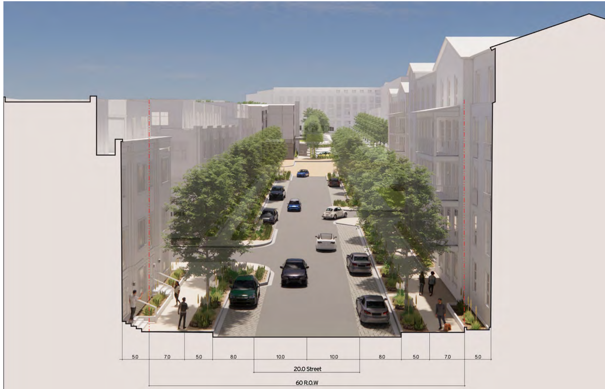
Figure 3-19 - New Local Street Section
