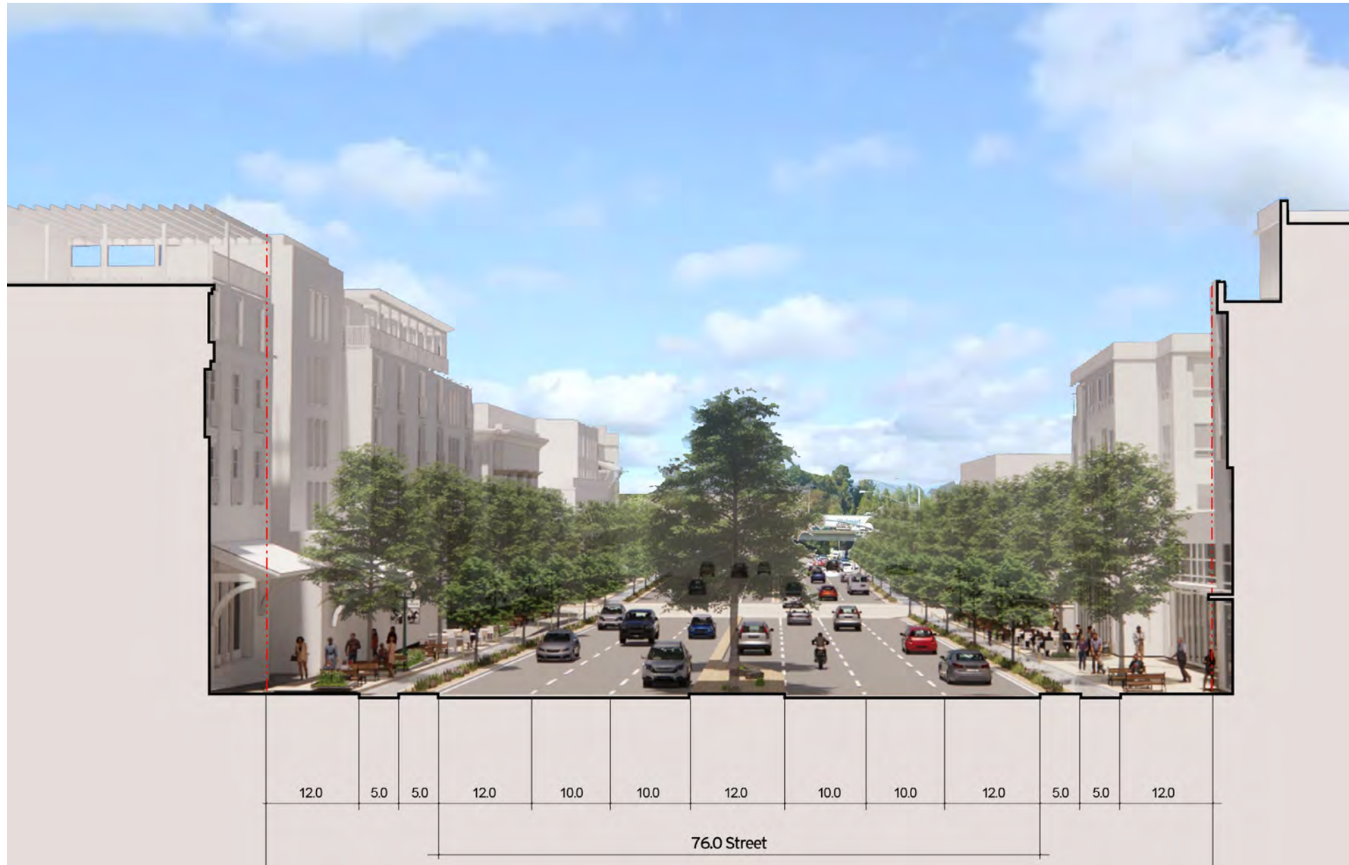
Figure 3-12 - Re-configured Diamond Bar Boulevard street section
